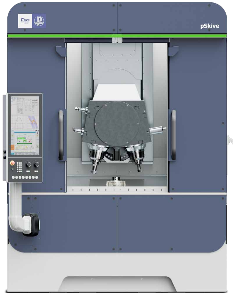
DUO head for two gear cutting tools
