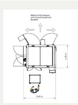
Cell expansion for loading and unloading using a forklift or AGV.
