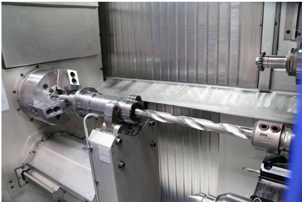
Deep hole drilling after pre-drilling
