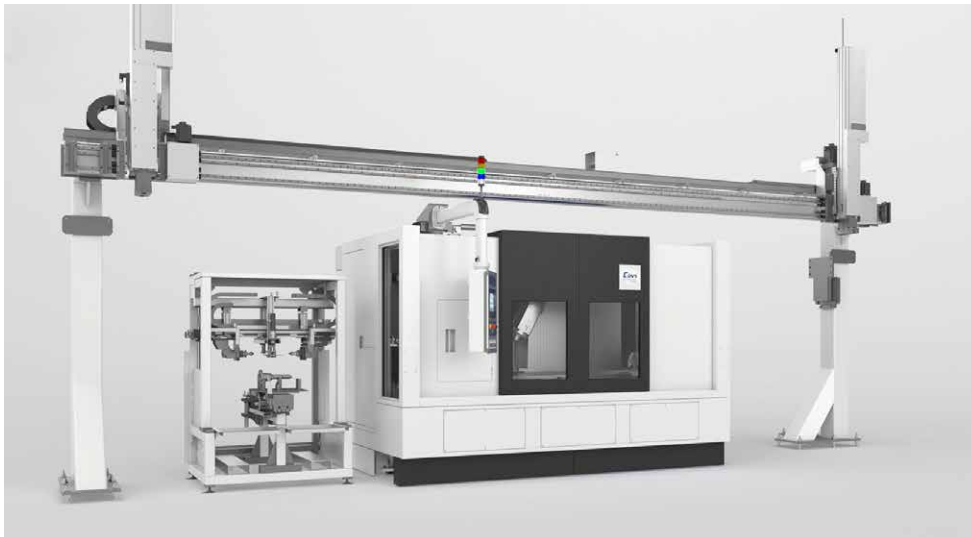
Machine with portal for top loading and external measuring station
